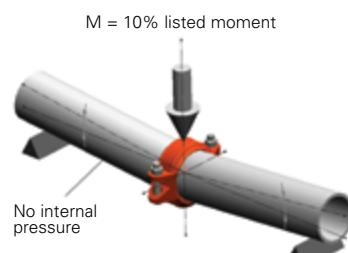
**Rigidity Proof Test** Rigidity proof testing is conducted by applying 25% of the listed moment to the test assembly which is internally pressurized to the rated pressure.
