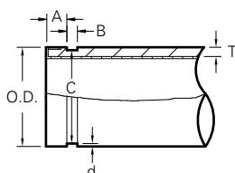
1. EP cut-grooves are for plastic coated or cement lined pipe to be connected with Shurjoint XH-70EP couplings only. Do not roll groove pipe, which can damage the coating or lining and or create flared pipe ends.
