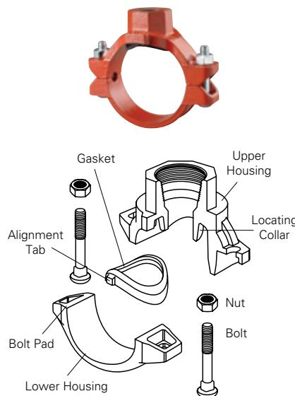
When bolts are tightened with a proper torque, the outlet housing makes metal to metal contact with the outer surface of the pipe.
