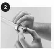
Slide nut over tubing, place retainer ring leaving one corrugation exposed.
