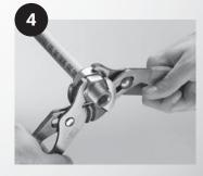
Tighten with wrenches until nut contacts body.
