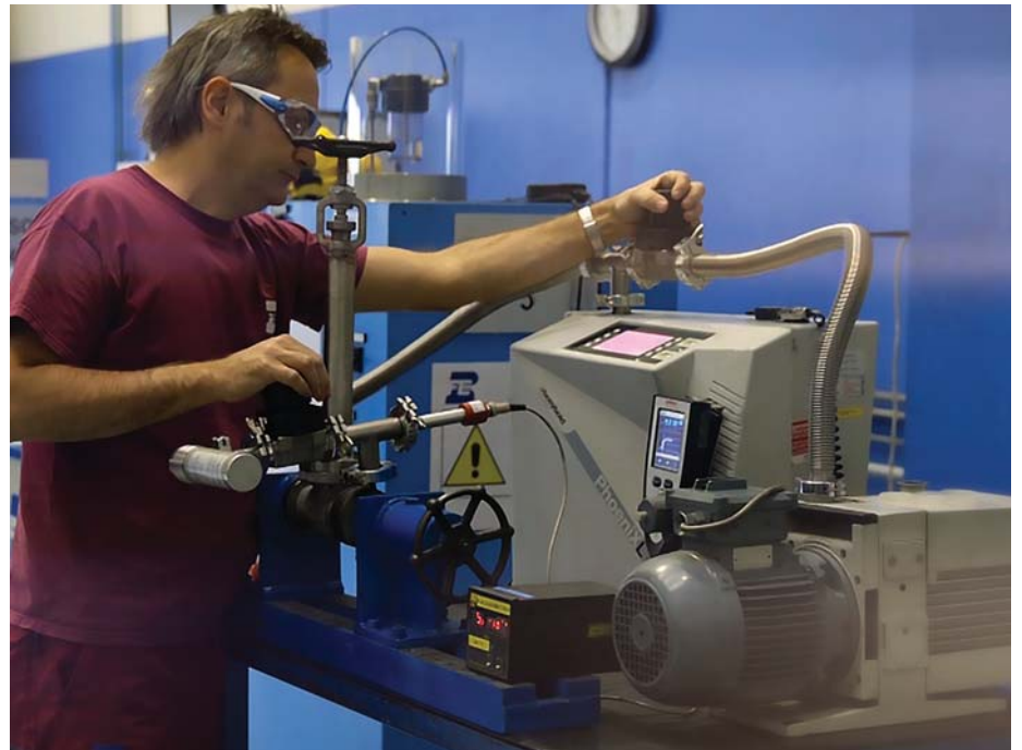
“Compliance Guaranteed”: Shown - Helium seat leak testing being performed. From steel microstructure testing to valve functionality testing BFE can provide it all.
