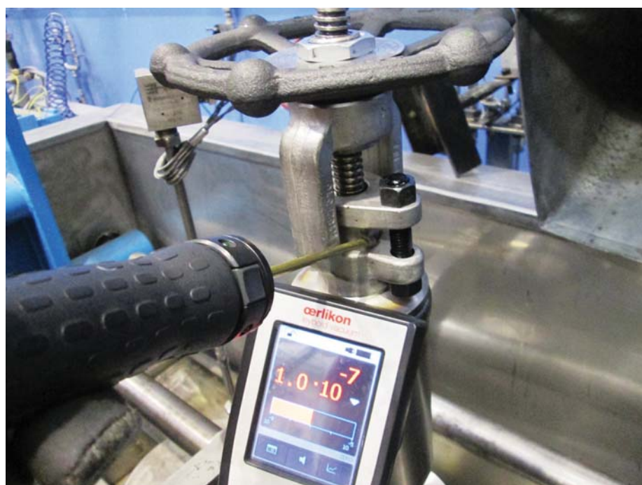
"The Low Emissions Leader": In-house, certified low emissions testing being performed on a gate valve – whether its API 624, ISO 15848 or more stringent emissions testing – BFE can do it.
