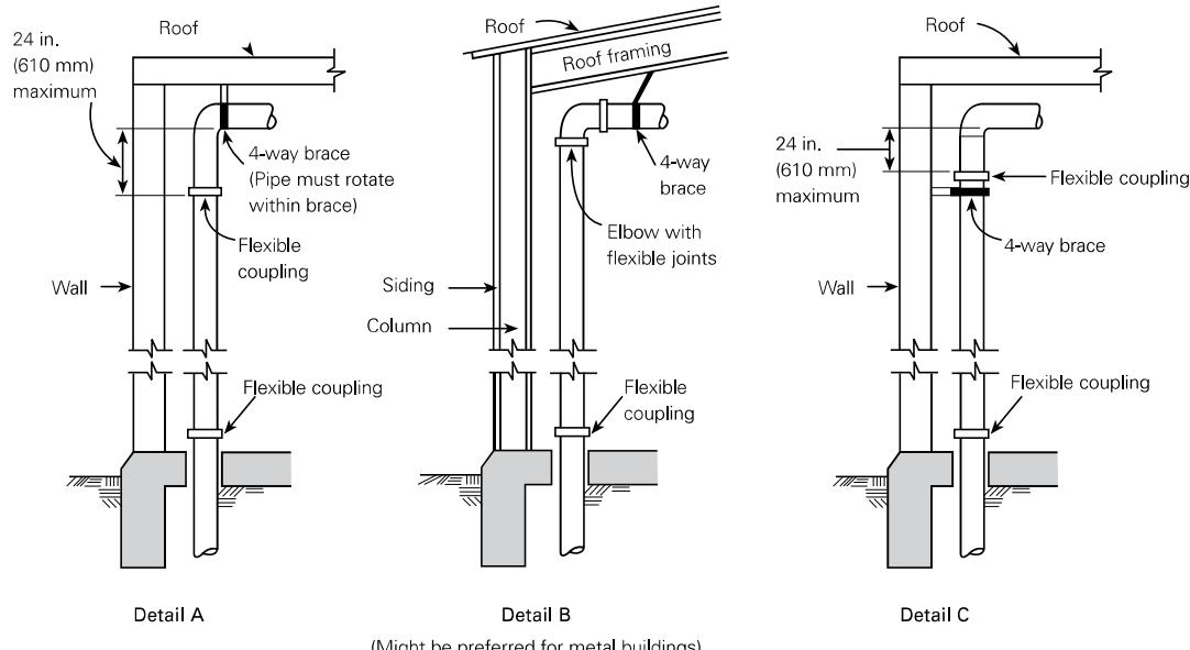
Note to Detail A: The four-way brace should be attached above the upper flexible coupling required for the riser and preferably to the roof structure if suitable. The brace should not be attached directly to a plywood or metal deck.
