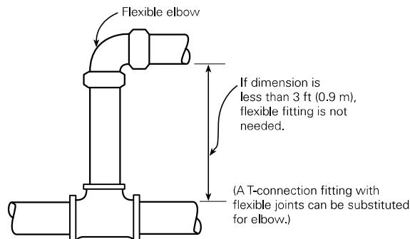
FIGURE A.9.3.2(b) Detail at Short Riser.
