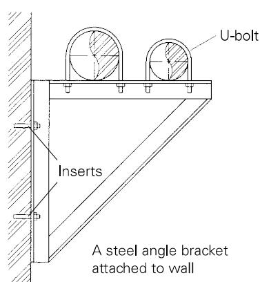
A steel angle bracket attached to wall
