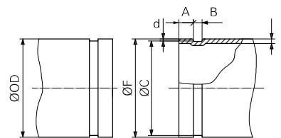
Figure 1 - Roll grooved-end dimensional reference points for Table 1
