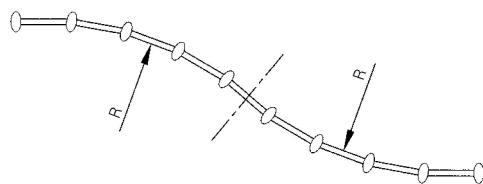
Example: When using model 7705 100 mm (4") couplings for the layout as shown in the diagram, the max. allowed deflection ( $\theta$ ) of the coupling is 3.4°, and the pipe length (L) is 5.5 meters, the radius of curvature (R) will be 92.7 meters.
