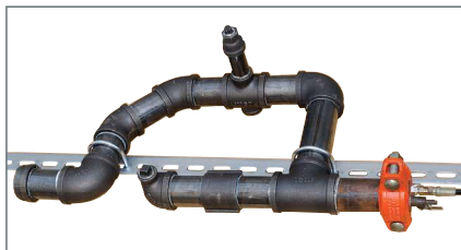
Burst pressure testing of DI threaded fittings (2")
