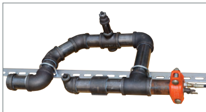
Burst pressure testing of DI threaded fittings (2")
