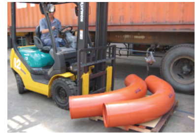
12" 3D 90° elbows ready for shipment
